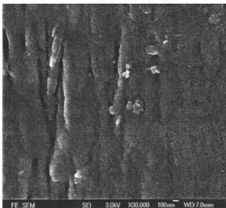
**Figure 9** SEM image of MMT-treated fabric with no binder after 3 times of padding ( $\times 30,000$ ).
